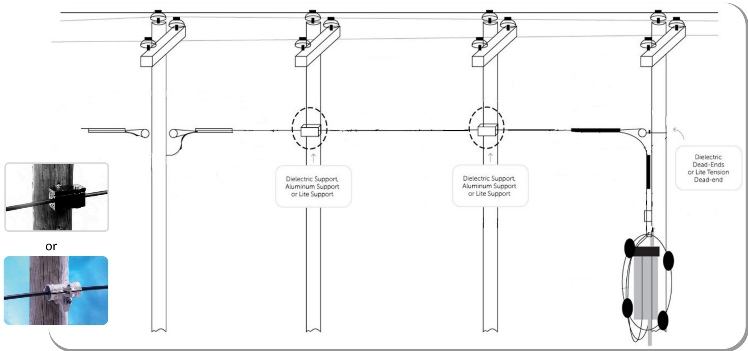
Supports create fixed points at each pole, so spans are mechanically independent
