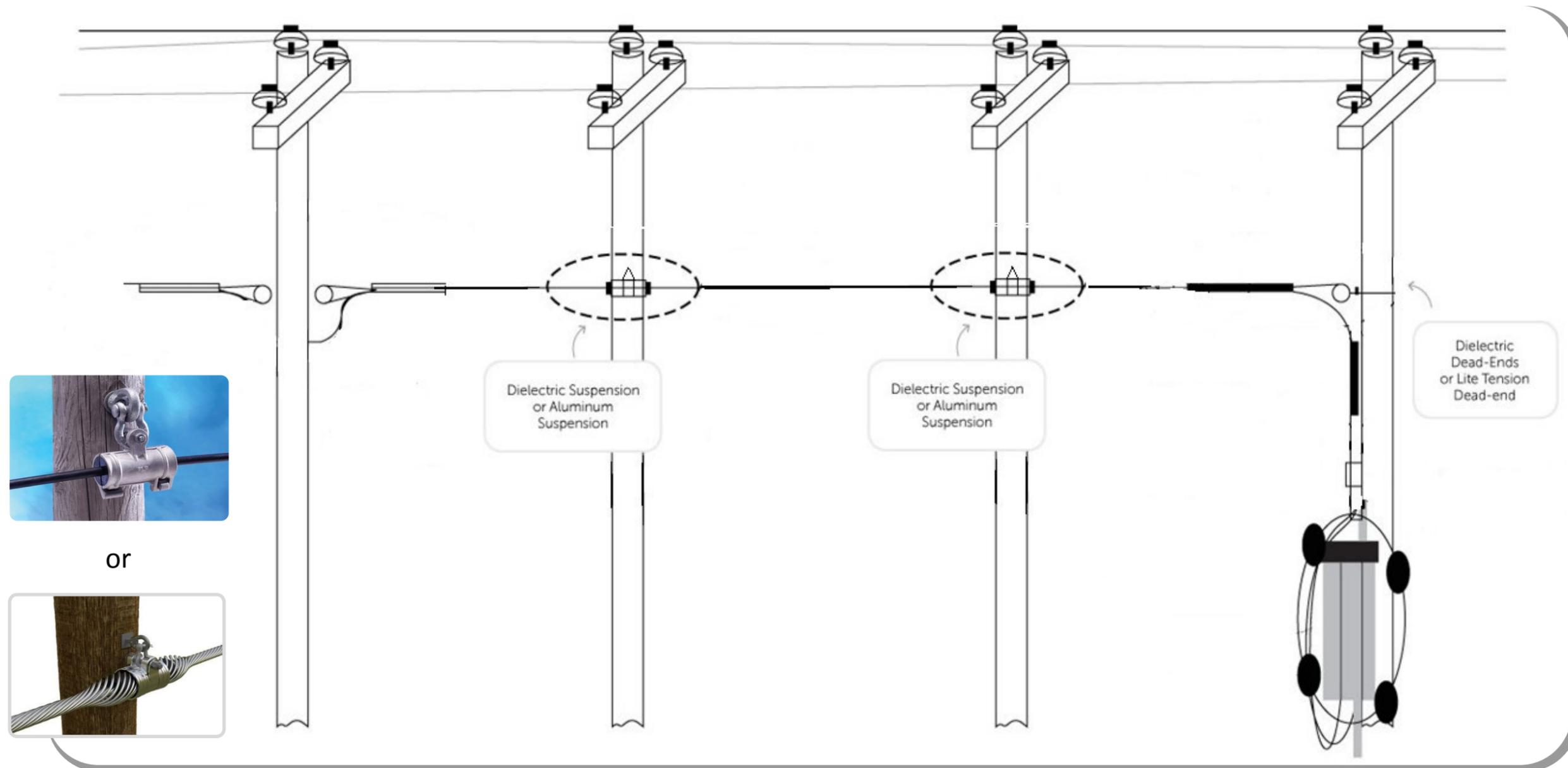
The articulation of a suspension clamp makes the spans mechanically coupled
