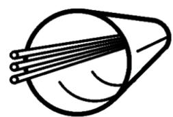
Defined stiffness to provide maximum blowing length (Use of different outer jacket material and central strength member)
