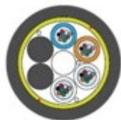
**This type cable is literally wrapped around an existing groundwire (or conductor)**
