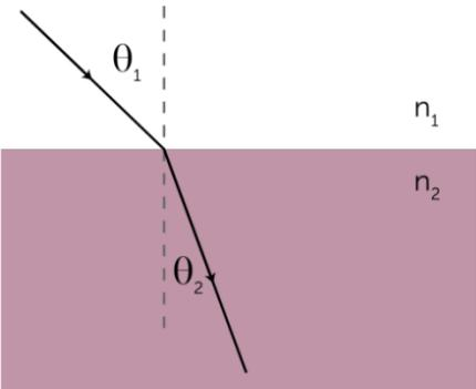
Light bends towards the normal when going from a medium with a smaller index of refraction to a larger index of refraction. (Light will have the smaller angle in the medium with the greater index of refraction).
