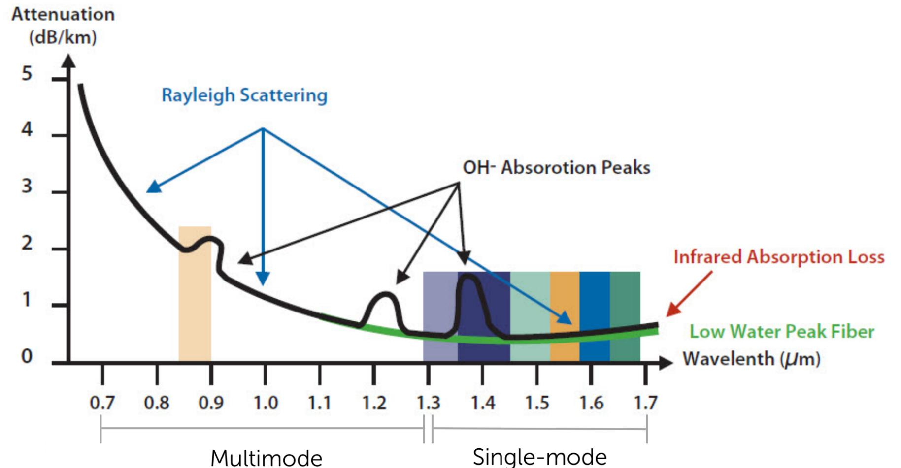
Fiber attenuation as a function of wavelength
