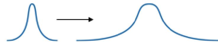
As a pulse travels down a fiber, dispersion causes pulse spreading. This limits the distance and the bit rate of data on an optical fiber.
