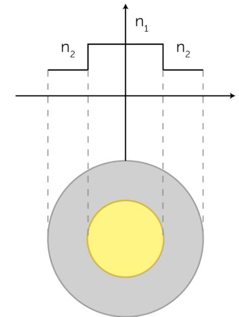
Refractive index of the medium = [Speed of light in a vacuum / Speed of light in the medium]
