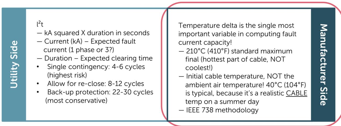
**Now we will see how a cable designer computes the fault current capacity for a cable design**
