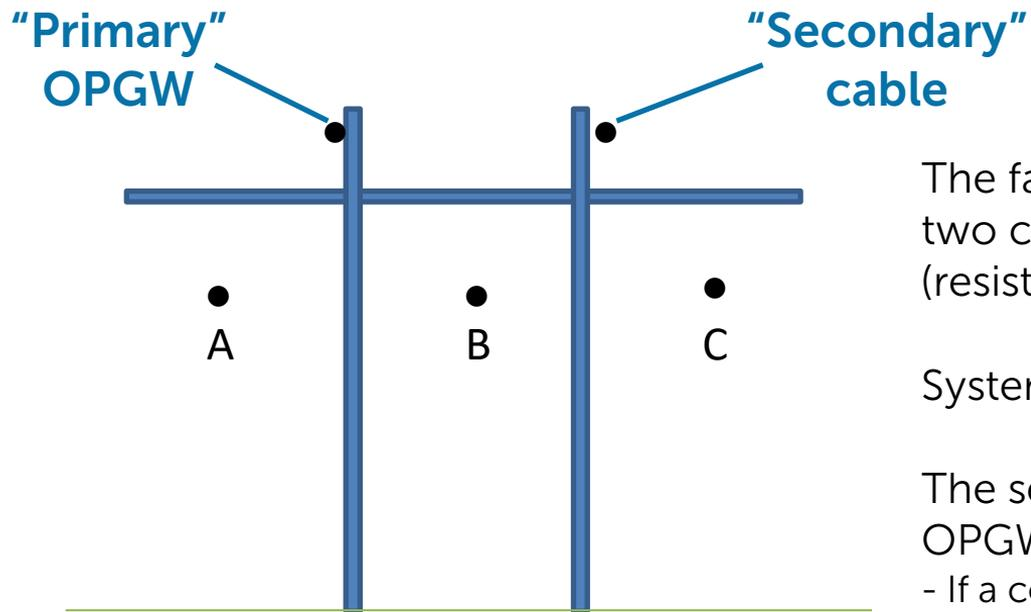
The fault current will divide between the two cables based on relative resistance (resistance in parallel)
