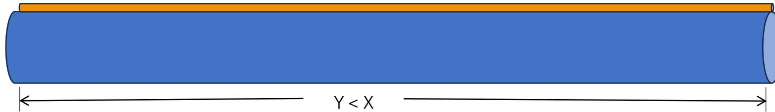
A higher temperature or increased wind or ice loading will cause the cable and fiber to stretch:
