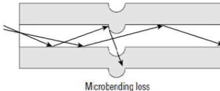
Resulting indentation impedes light transmission in both fibers
