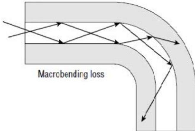
Light is not being reflected internally; it is "escaping" which equates to signal loss
