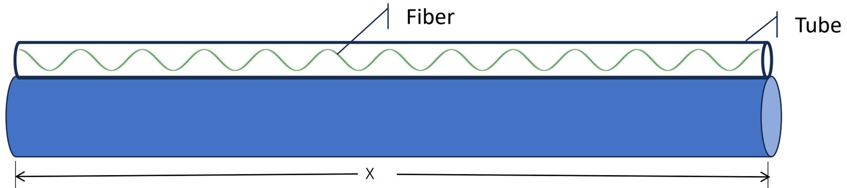
That is:  $L_{\text{fiber}} > L_{\text{tube}}$
