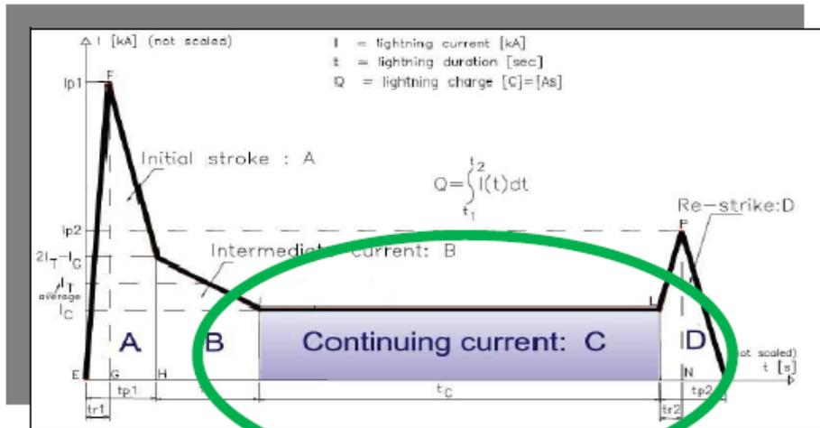
Fig. 1 Conventional waveform of current in a lightning discharge<sup>1</sup>
