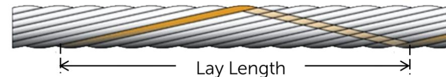
Distance required to complete 1 revolution of a tube around the diameter of what's underneath (typically, the center element)
