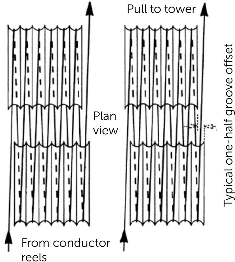
Notice that the **conductor** is going **left to right** and that the **offset** of the front set of wheels is to the **left** relative to the back set
